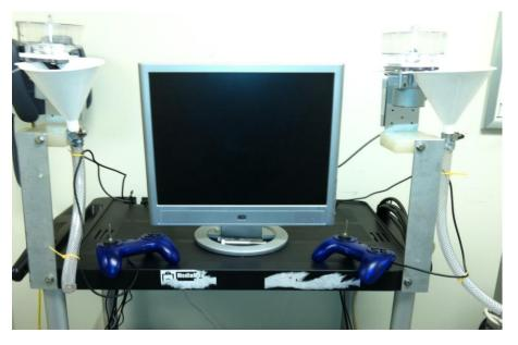
*Figure 1.* Joint computerized apparatus used for testing. Pairs of monkeys shared one computer screen but had their own joystick that would attach to their testing box and pellet dispenser.
